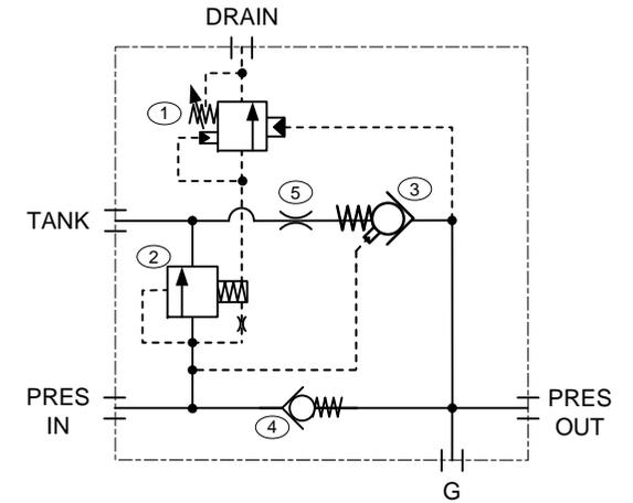
NOTE: Maximum pressure with this setup is limited to 2000psi. Higher pressures may be achieved by using a heavier spring tension in the unloading element (2)
